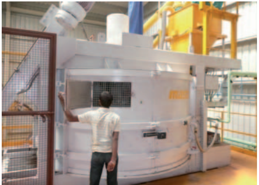
Two concrete mixers by Masa produce the facing and core concrete for the block production
